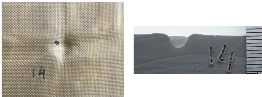
Fig. 2. Deformation of two layers of the fabric of plain weave P110 with PVA treatment and technical plasticine after the local impact
