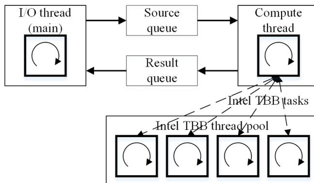
**Fig. 2.** The block diagram of the data processing application for the supercomputer.
