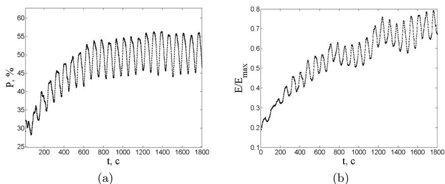
**Fig. 6.** a – temporal variation of the heating power (percentage of the maximum value); b – temporal variation of the kinetic energy of azimuthal flow in the heating area.
