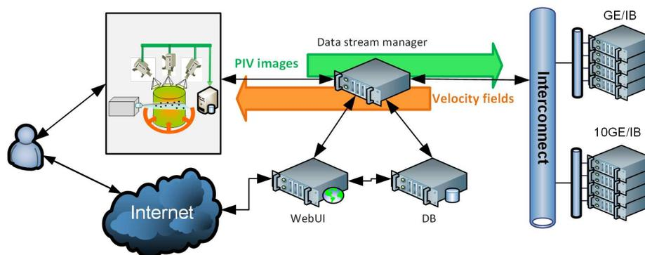
**Fig. 1.** The architecture of a system for processing experimental data on a supercomputer
