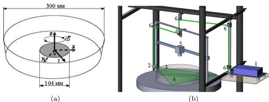
**Fig. 4.** Experimental model, dimensions and location of the coordinate system (a); experimental stand (b): 1 – dual pulsed laser for PIV, 2 – laser sheet system, 3 – laser sheet, 4 – tracers, 5 – CCD camera, 6 – mirrors.
