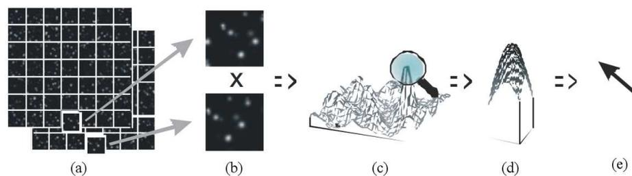
**Fig. 3.** The stages of operation of PIVlab software: a – formation of interrogation windows, b – cross-correlation, c – search for correlation maxima, d – determination of the coordinates of the maxima, e – calculation of the velocity vector.
