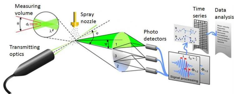
Fig. 8. Optical scheme for analysis of particle dynamics (Particle Dynamics Analysis).
